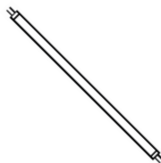
Watts: 8W / 13W FLUORESCENT T5 G13 BI-PIN BASE Ballast: BLST08-T5 JTS-8 JTS-13
