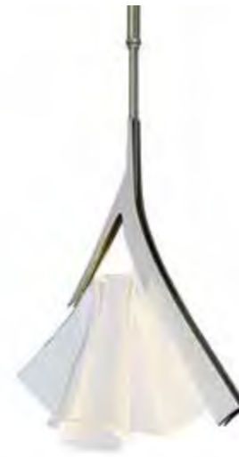
MOBIUS LED PENDANT - 139845 11.7" h x 8.4" w x 4" d - 5.5" OD canopy - 50" wire - 3.8 lbs 300 EST. DELIVERED LUMENS, 7W, 3000K CCT, 90 CRI, 120-277V AC INPUT, 0-10 ELV DIMMING
