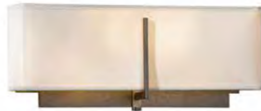
EXOS SQUARE SCONCE - 207680 6.8" h x 16.5" w x 4" d - 6 lbs 15.8" x 5.5" backplate - 4" vertical mounting ht Candelabra sockets (2), 15 W max, B LED bulbs
