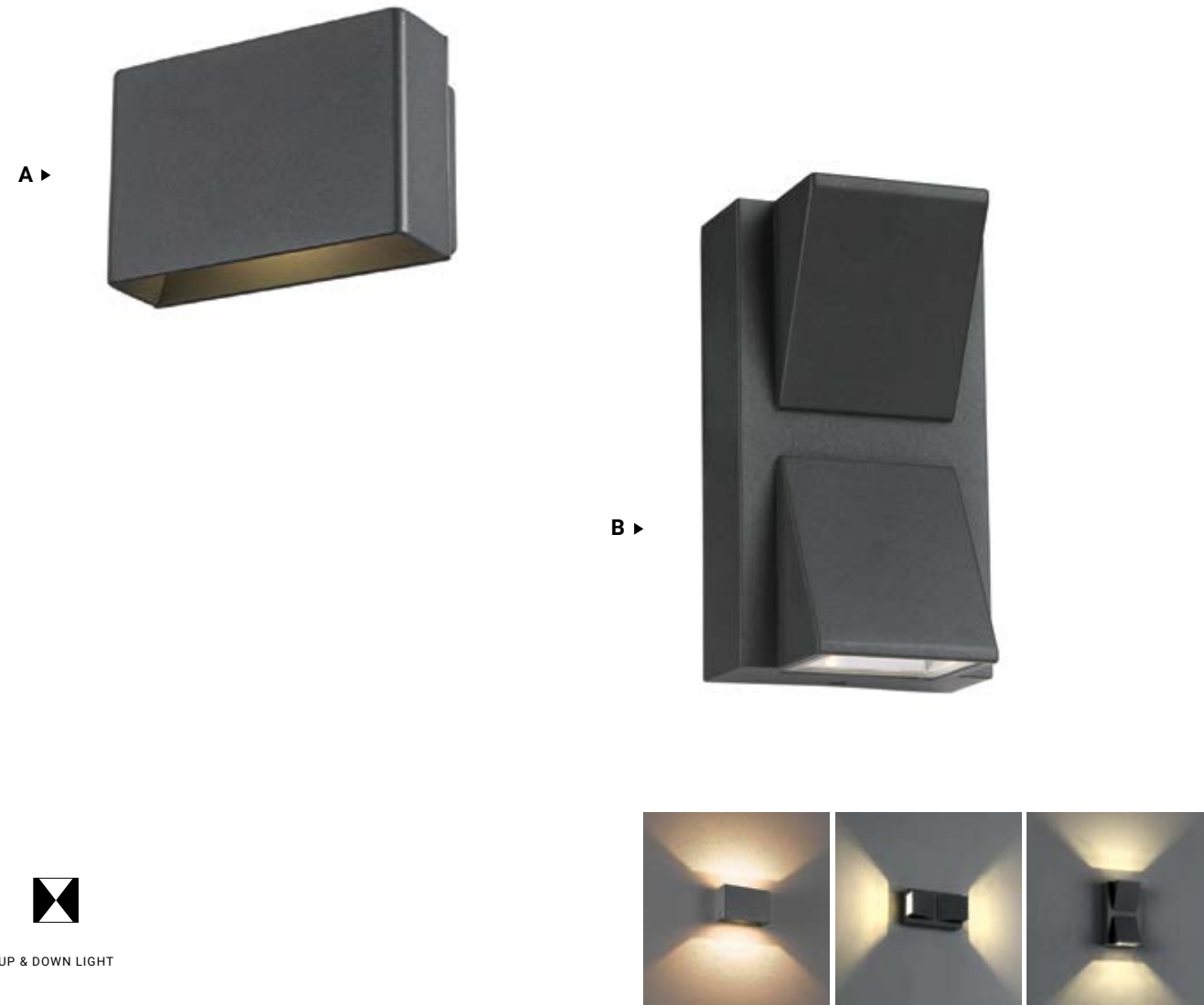
A 28282-020 LED LED Wall Mount W: 4.75" | H: 3.25" | EXT: 2.25" 1 x 5W LED 3000K 150 Delivered Lumens 80+ CRI Dimmable Wet Rated IP54
