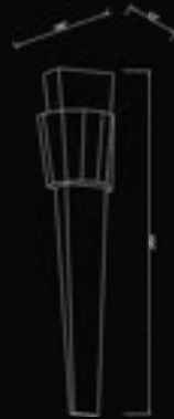
HF3011-PN 7"W x 22"H x 4"EXT 9W/120V LED 770lm 3000K Dimmable Clear Crystal
