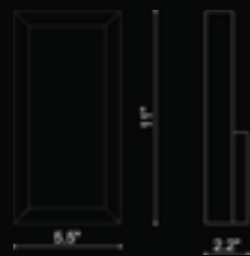
HF6015-BA Brushed Aluminum 5.5" W x 11"H x 2.2" Ext 12 Watt 120 Volt 800 Lumens 3000K
